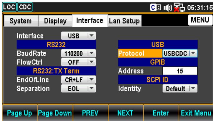
5. Press the F5 (Enter) key or Knob key followed by scrolling Knob key or pressing +/- keys to land on the desired USB Protocol option. We adopt USB-CDC in the example here.
