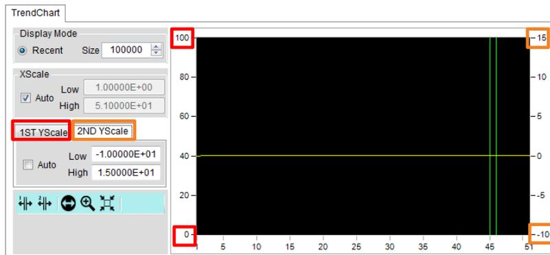
Note The 2ND Y Scale section hides out when the 2ND display measuring function is disabled.
