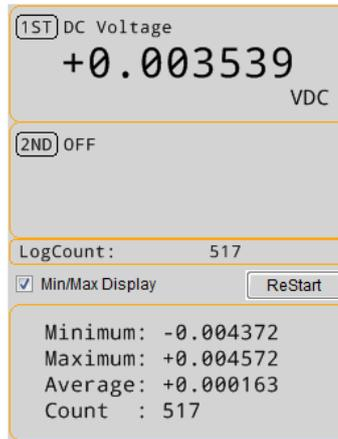
When the 2ND display is enabled, the measured value will be shown in 2ND section and the **Min/Max Display**, however, will be deactivated.
