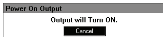
Figure 4-25 The Message Window to be Shown Before the Automatic Output-On After the Power-On
