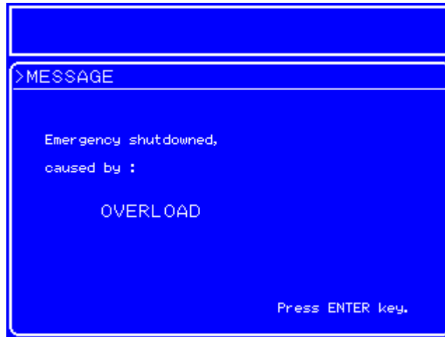
Figure 6-1. Protective Function Related Error Display Examples
