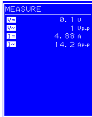
Figure 4-31. Measurement Value Display Example
