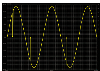
Commutation notch (thyristor controlled noise simulation)
