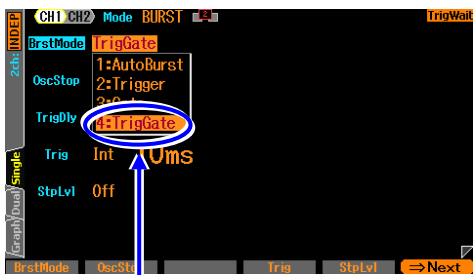
Select [TrigGate] on the burst mode setting menu
