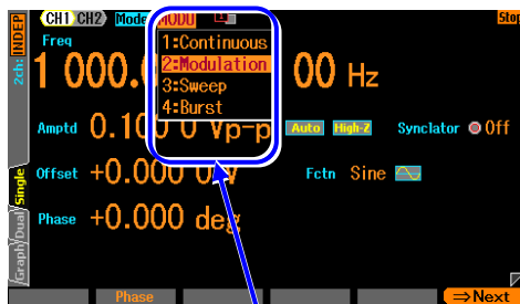
Set the oscillation mode to [Modulation]
