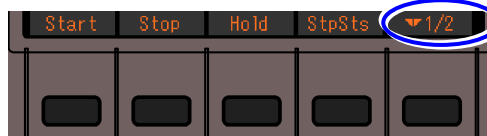
Indicates that the first of two stages of soft-keys is displayed. When this key is pressed, the soft-keys for the next stage is displayed.
