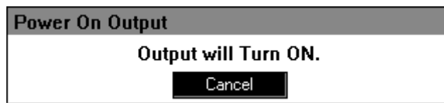
Figure 4-26 The Message Window to be Shown Before the Automatic Output-On After the Power-On
