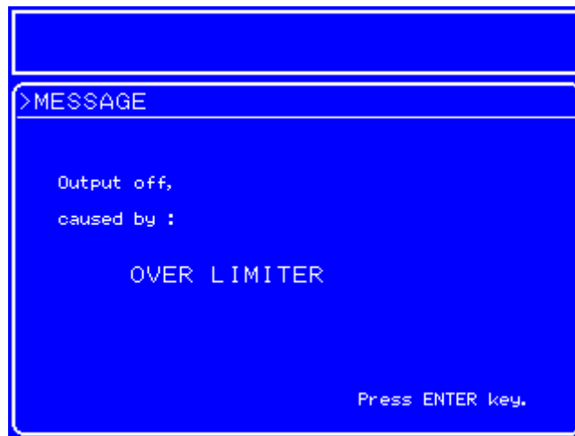
Figure 6-3. Warning Display Example
